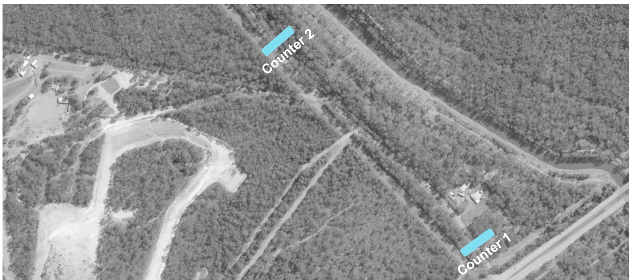
Figure 2.2 Tube counter locations
